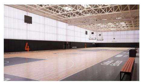
panels also included a softlite (anti-glare) layer to mitigate any dazzle due to bright sunlight during the day or strong artificial lighting at night.
